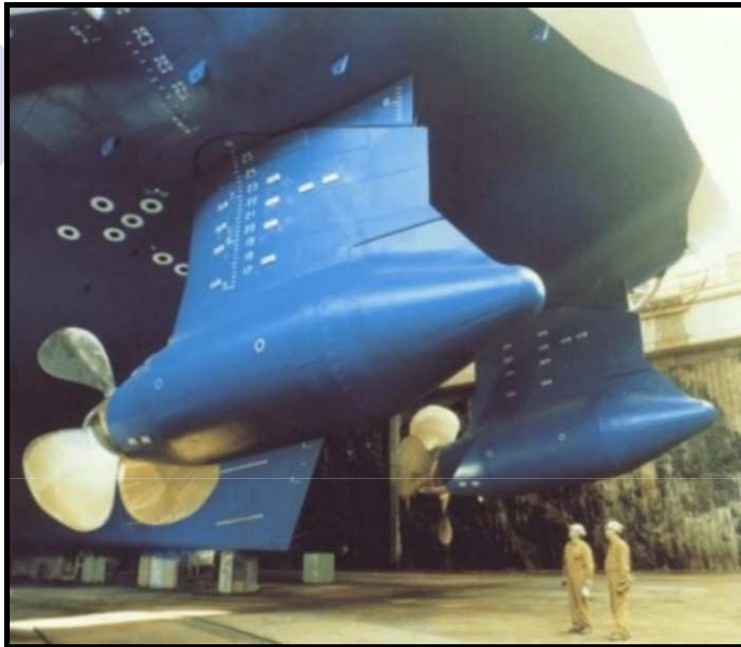
2 x 14MW Synchronous Motors ...apparently, they use permanent magnets!
